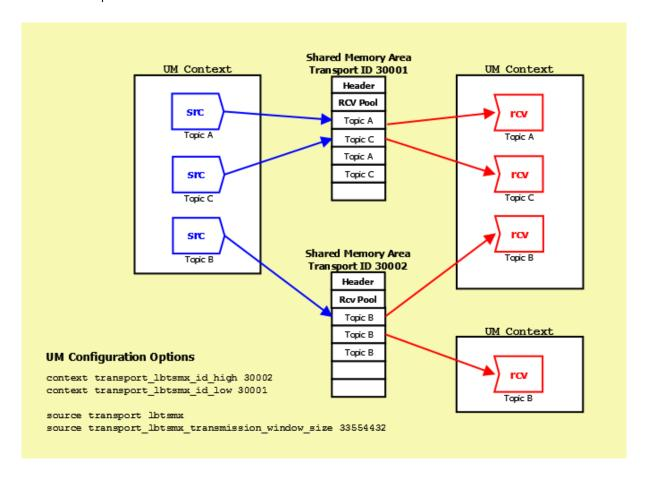
In the diagram above, three sources send (write) to two Shared Memory Areas while four receivers in two different contexts receive (read) from the areas. The assignment of sources to Shared Memory Areas demonstrate UM's round robin method. UM assigns the source sending on Topic A to Transport 30001, the source sending on Topic B to Transport 30002 and the source sending on Topic C back to the top of the transport ID range, 30001.
