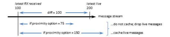
The default value of this option is high enough to still encourage caching most of the time, and should be optimal for most receivers.
