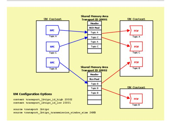
In the diagram above, 3 sources send (write) to two Shared Memory Areas while four receivers in two different contexts receive (read) from the areas. The assignment of sources to Shared Memory Areas demonstrate UM's round robin method. UM assigns the source sending on Topic A to Transport 20001, the source sending on Topic B to Transport 20002 and the source sending on Topic C back to the top of the transport ID range, 20001.
