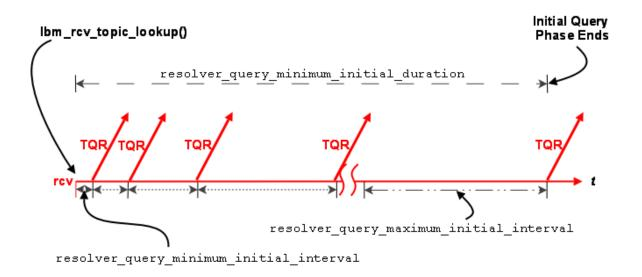
The initial query phase completes when it reaches the **resolver\_query\_minimum\_initial\_duration (receiver)**. The initial query phase also has UM context-wide rate limit controls (**resolver\_initial\_queries\_per\_second (context)** and **resolver\_initial\_query\_bps (context)**) that can result in the extension of a phase's duration in the case of a large number of topics or long topic names.
