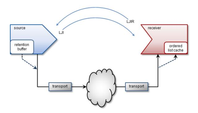
The source's retention buffer's is not pre-allocated and occupies an increasing amount of memory as the source sends messages and adds them to the buffer. If a retention buffer grows to a size equal to the value of the source configuration option, retransmit\_retention\_size\_threshold (source), the source deletes older messages as it adds new ones. The source configuration option retransmit\_retention\_age\_threshold (source), controls message deletion based on message age.
