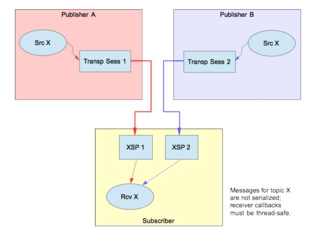
Publisher A and B are two separate application instances, both of which create a source for topic "X". A subscriber application might create two XSPs and assign one transport session to each. In this case, you have two independent threads delivering messages to the subscriber's receiver callback, which may not be what the developer wanted. If the developer wants topic X to be serialized, a single XSP should be created and mapped to both transport sessions:
