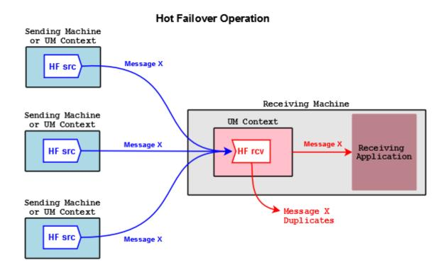
In the figure above, HF sources send copies of Message X. An HF receiver delivers the first copy of Message X it receives to the application, and discards subsequent copies coming from the other sources.
